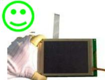
As above picture, please handle with anti-static gloves around LCM edges.
